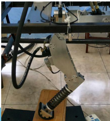
Figure 12 Structure of the single leg of hydraulic quadruped robot
